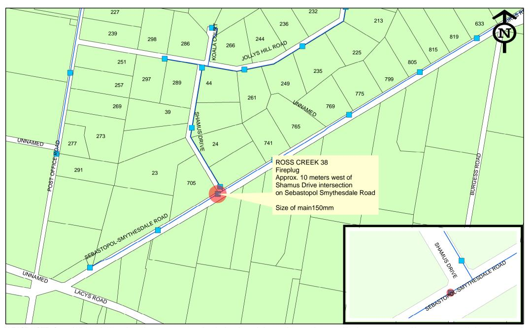
PLEASE NOTE: Central Highlands Water has taken care to ensure that the locations of pipes and assets shown on this plan are accurate. However, some variations from records do exist and complete accuracy cannot be guaranteed. In all instances it is essential that the position of the pipes concerned be proved on site by field survey and hand excavation. It is an offence to destroy, alter or in any way interfere with any works or property of CHW (Water Act, 1989 Section 288).
